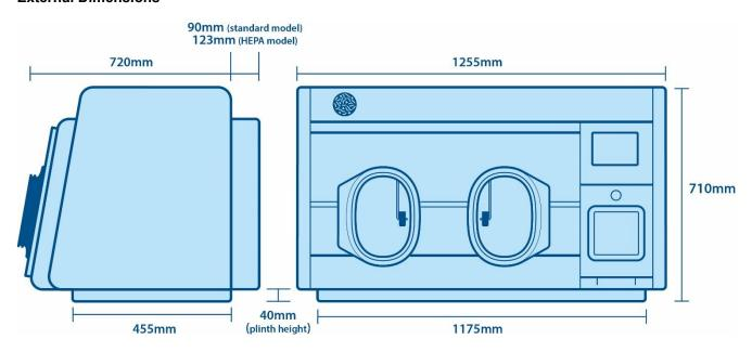
**Important note:** The HEPA model has a 123mm protrusion covering the entire rear of the chamber. The non-HEPA model has a localised protrusion of 90mm behind the airlock to accommodate condenser bottle, bracket, gas and electrical supplies. If bench mounted, a further minimum clearance of 500mm is required both above and at the right-hand side of the workstation for user/service access.
